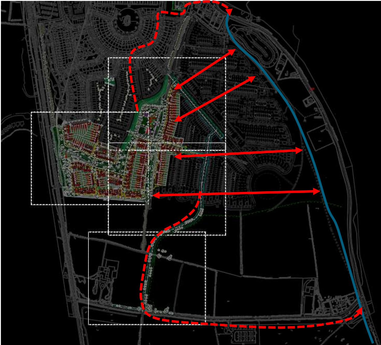
Figure 2.13.1 Portmarnock Greenway (blue) and the potential unsafe routes vulnerable road users might take (dashed red arrows) in the absence of direct connections (red arrows)
