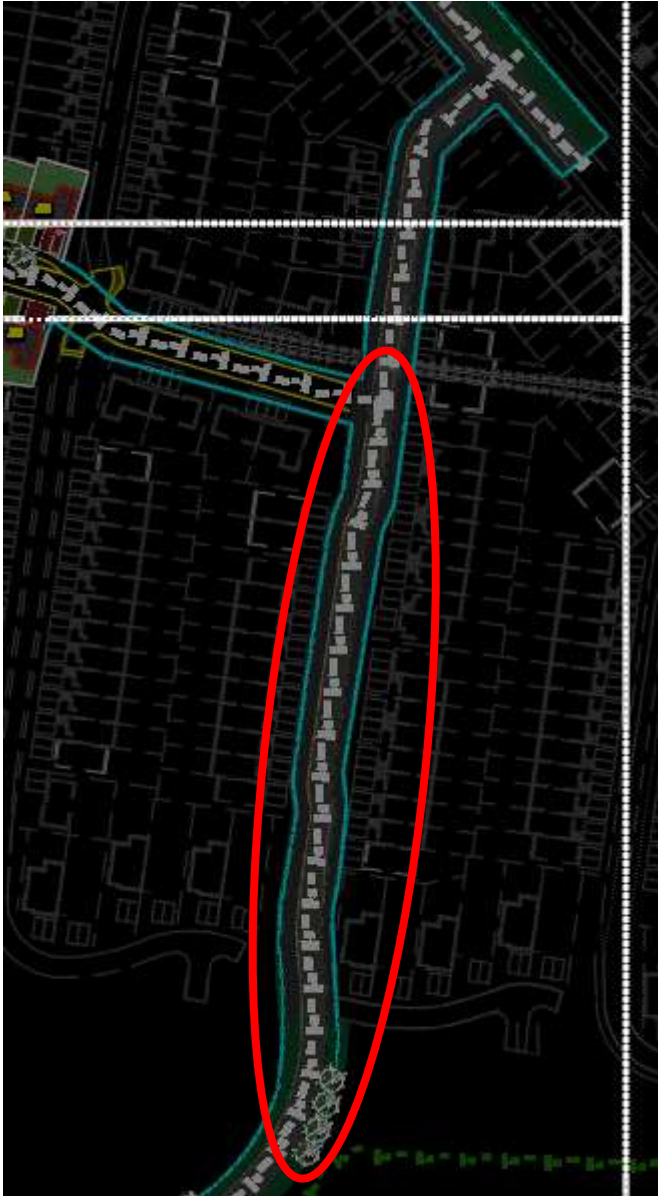
Figure 2.15.1 Bends and kinks in the alignment that may not be expected by drivers in the interim scenario, and may be hard to see in darkness
