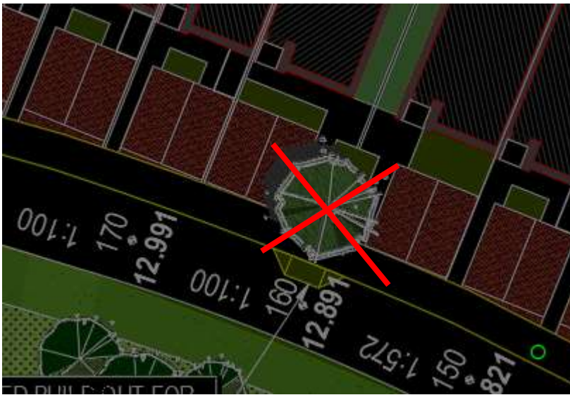
Figure 2.3.1 An example of a tree proposed between the parking spots that could obscure visibility and should therefore be removed from the proposals
