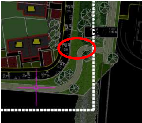
Figure 2.8.1 Lack of convenient connection to the cycle/pedestrian facility at the south-eastern end of the estate
