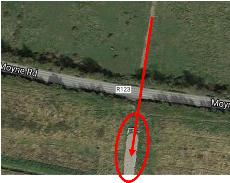
Figure 2.17.2 Aerial photo from before the access was constructed showing the existing road that could cause a see-through problem even if the access is blocked (source: Open-source aerial photography)
