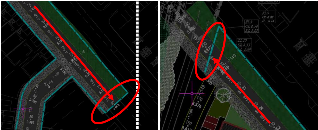
Figure 2.15.2 The fenced off extensions of the straight section of road that could mislead drivers in darkness
