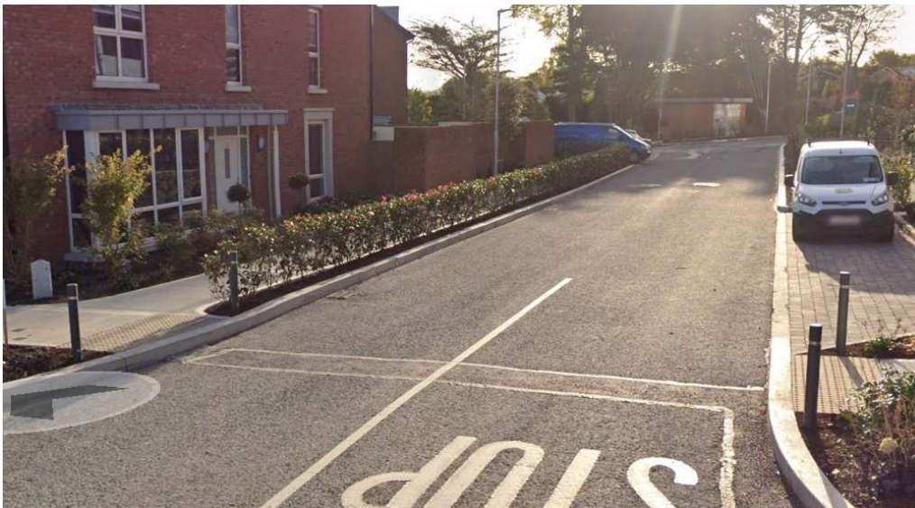
Figure 2.2.2 Examples of vegetation separating the footpath from the carriageway, also acting as a parking deterrent (source: Open-source street view photography)
